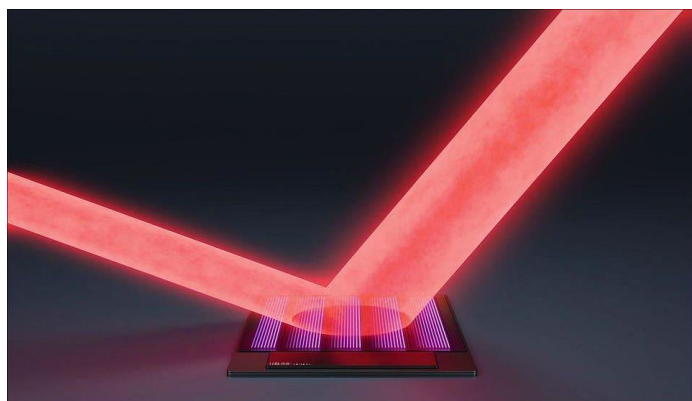
Figure 2: Metasurface (free-space) -- a sub-wavelength liquid-crystal pixel array imposes a programmable phase profile on the wavefront, steering the beam to a chosen output port [27].
