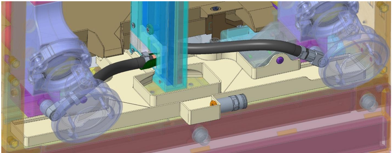
Figure 38: Manifold inlet/outlet connections shown. Nominal positions provided in 3D CAD. Drip/leak tray is also shown, in beige
