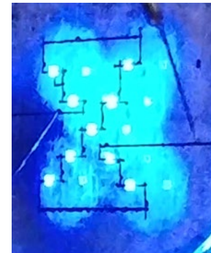
Printed LEDs (inkjet interconnects)
