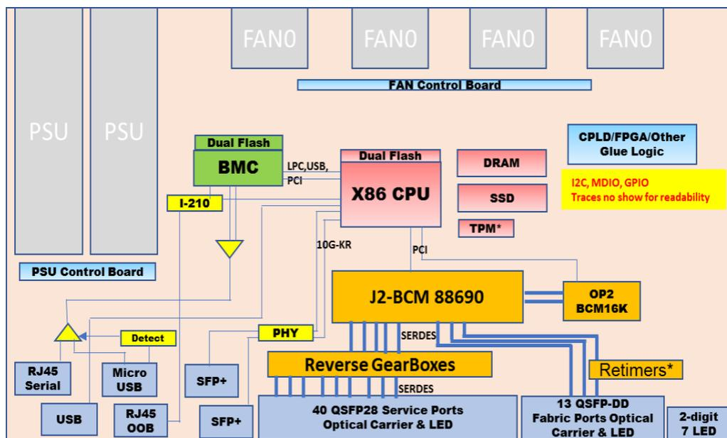
Figure 2: Architecture and Components of the NCP White-Box
