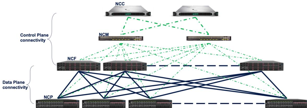
Figure 1: High-Level View of a Network Cloud platform
