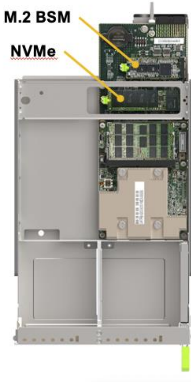
Figure 24: System Controller Module (SCM) top view
