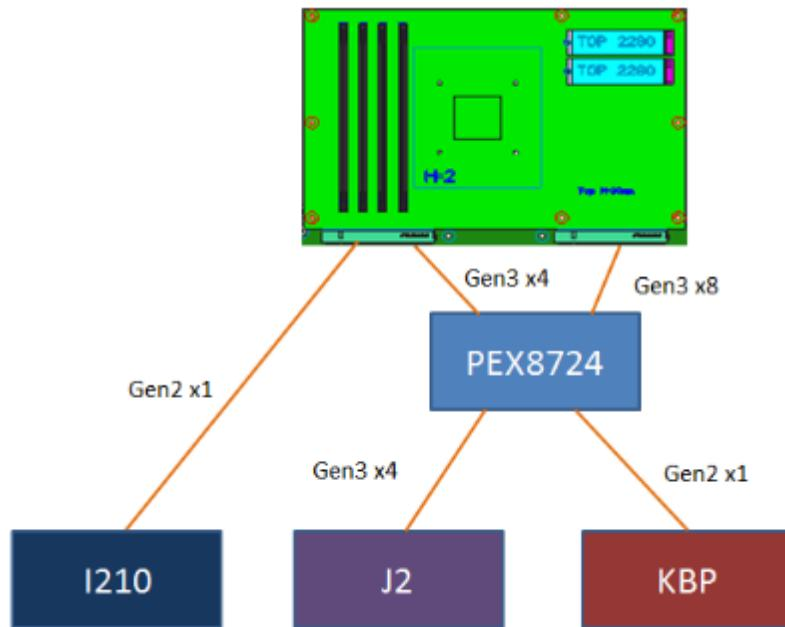
Figure 5-13 PCIe Connection Diagram
