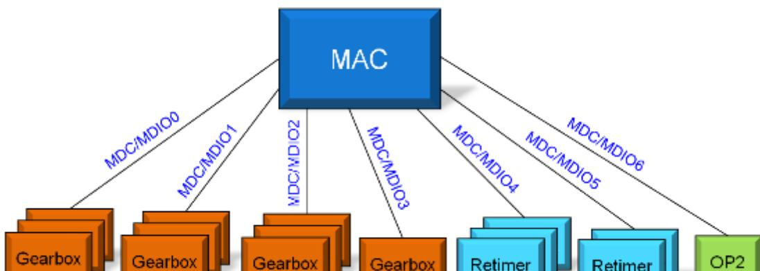
Figure 5-8 Physical Ports Assignment
