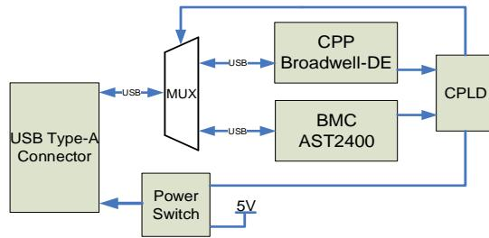
**Figure 5-21 USB Interface Diagram**
