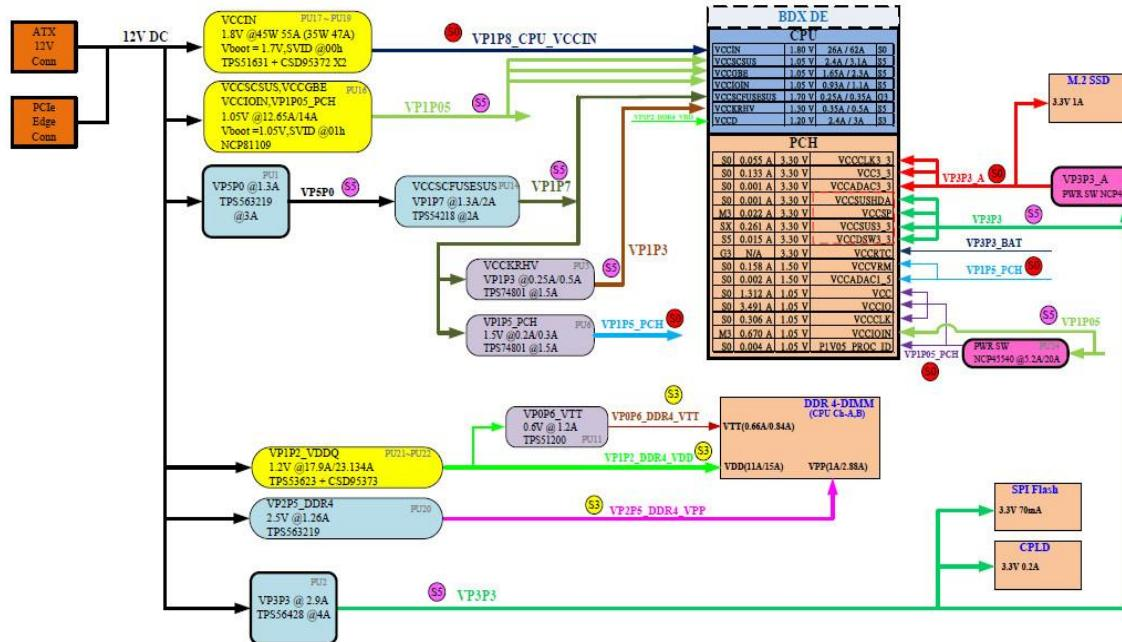
Figure 5-3 CPU Card DC/DC Power Distribution Diagram
