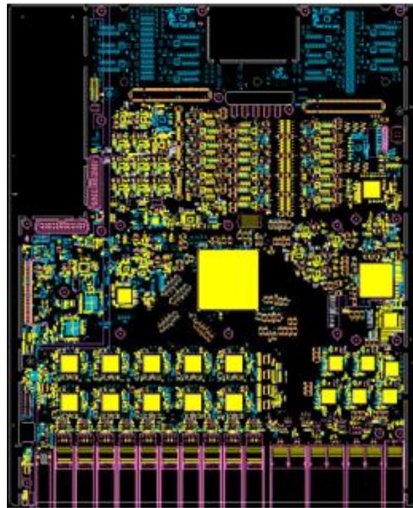
Figure 4-2 Switch Board PCB Layout
