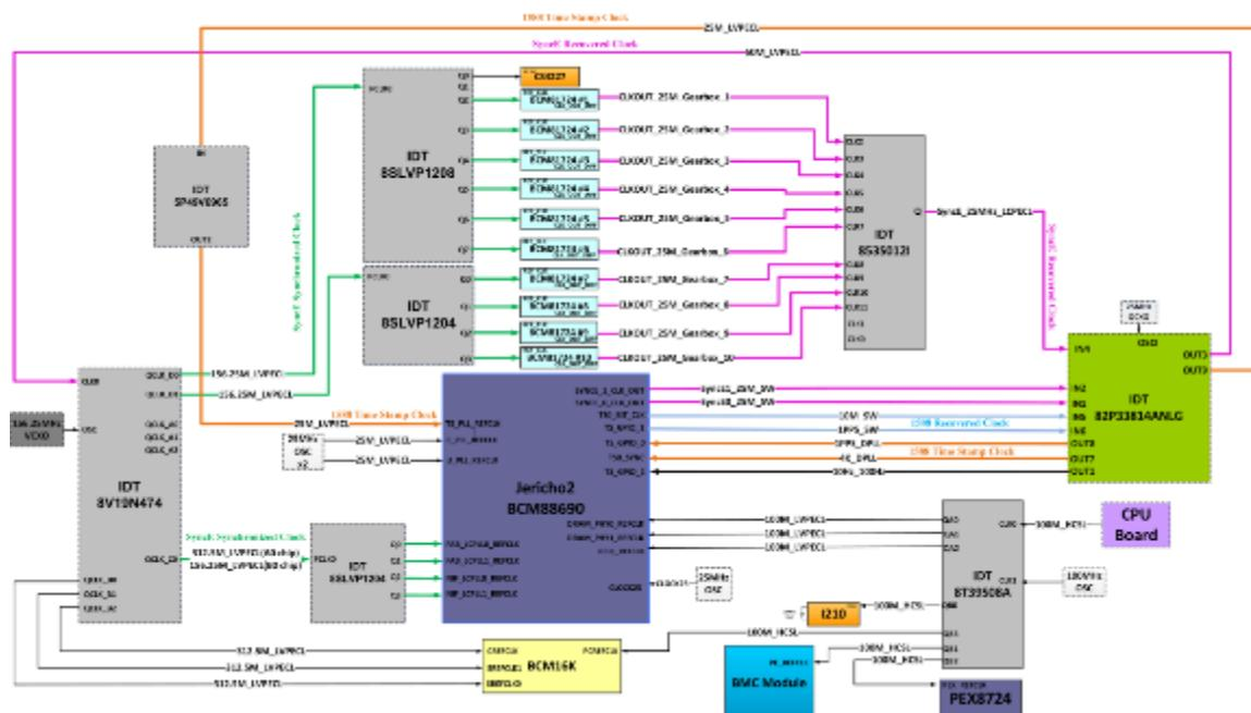
**Figure 5-11 S9700-53DX Switch Board Clock Diagram**
