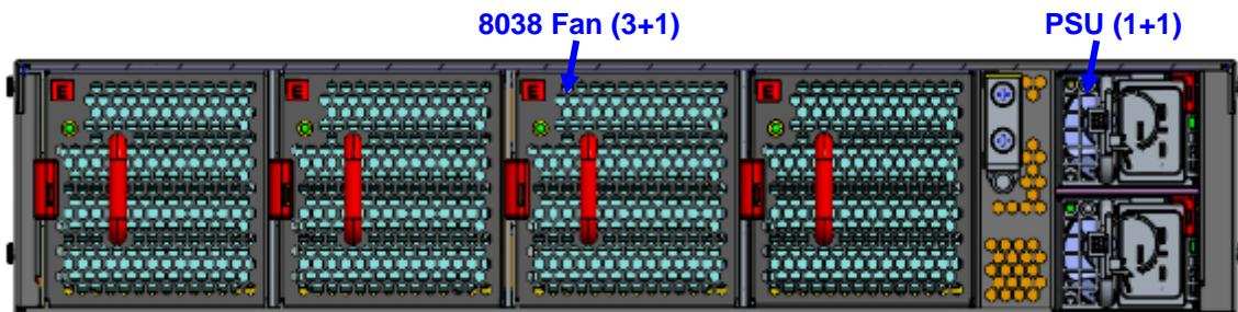
Figure 5-20 Rear Panel IO Arrangement
