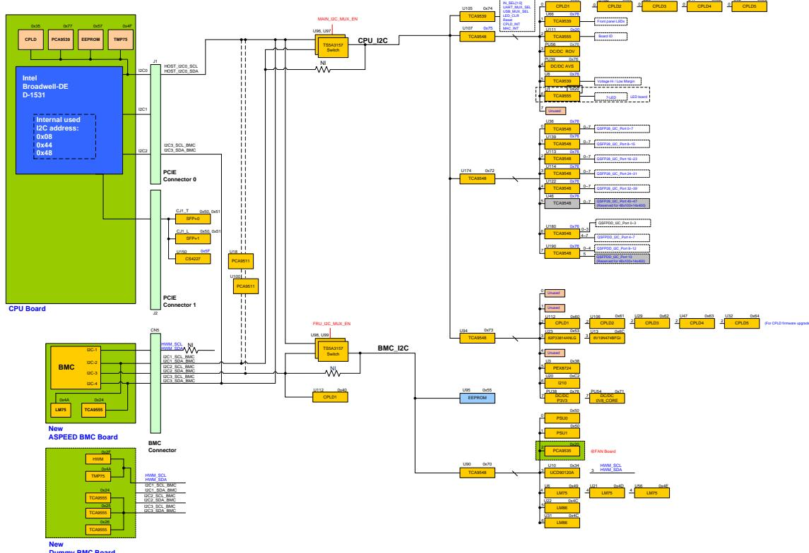
Figure 5-12 I<sup>2</sup>C Bus Connection Diagram
