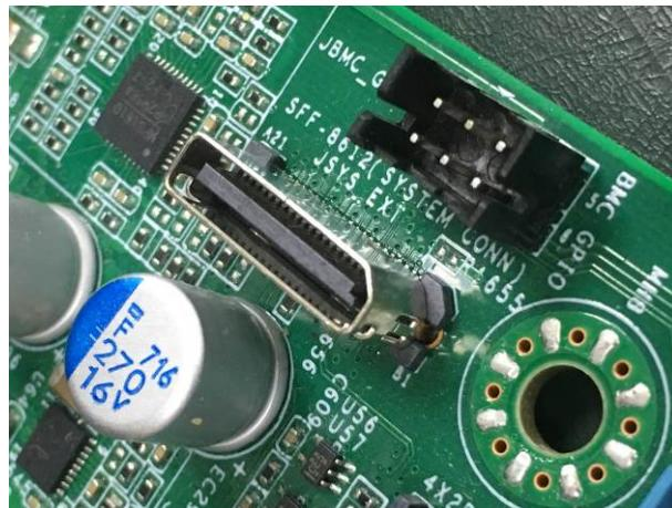
Figure 39 - SFF-8612 Connector on motherboard
