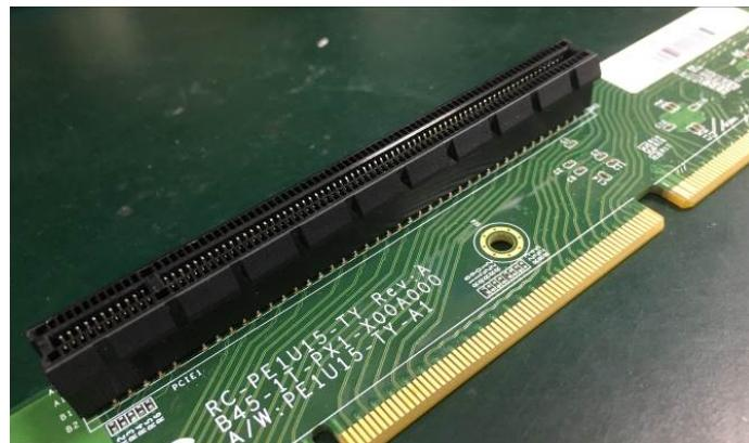
Figure 21 - PCIE x16 slot PCIE1
