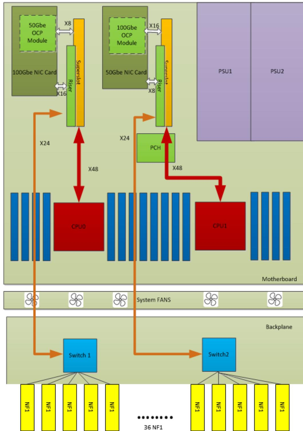
Figure 3 - Mission Peak System Placement Block Diagram
