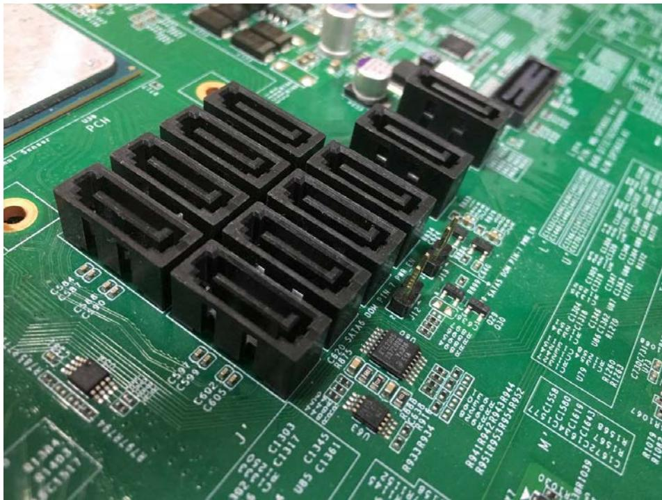
Figure 33 - Standard SATA Connector on motherboard
