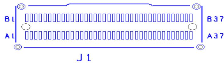
Figure 22 - Slimline Connector J1
