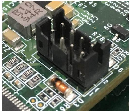
Figure 38 - Fan Connector
