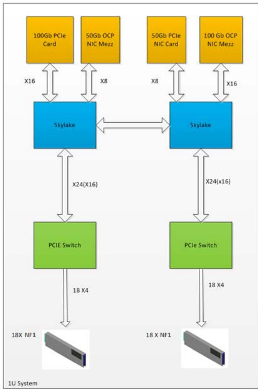
Figure 2 - NF1 (NGSFF) POC High-level System Block Diagram
