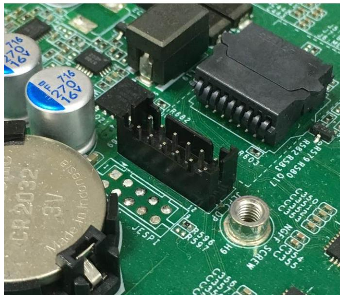
Figure 36 - JLPC Debug Header
