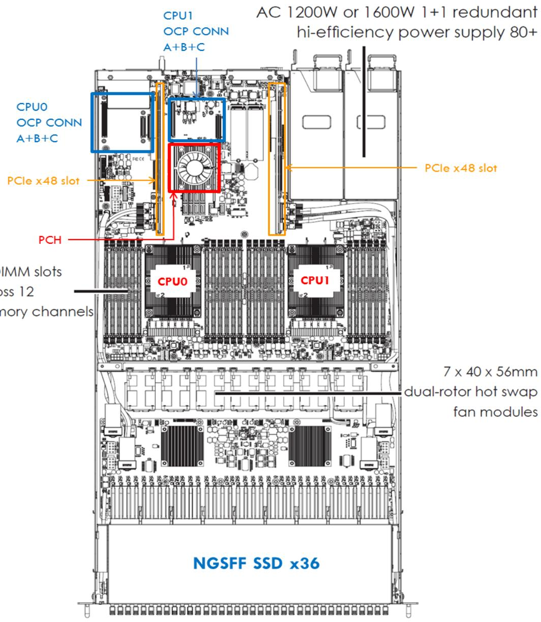
Figure 8 - Mechanical Placement
