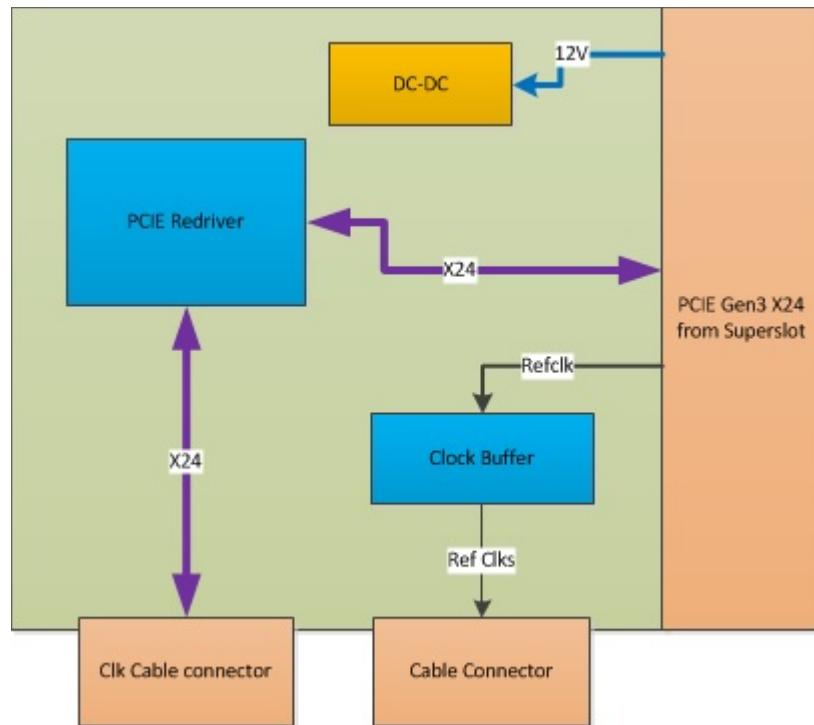
Figure 13 - NF1 (NGSFF) POC PCIe Riser
