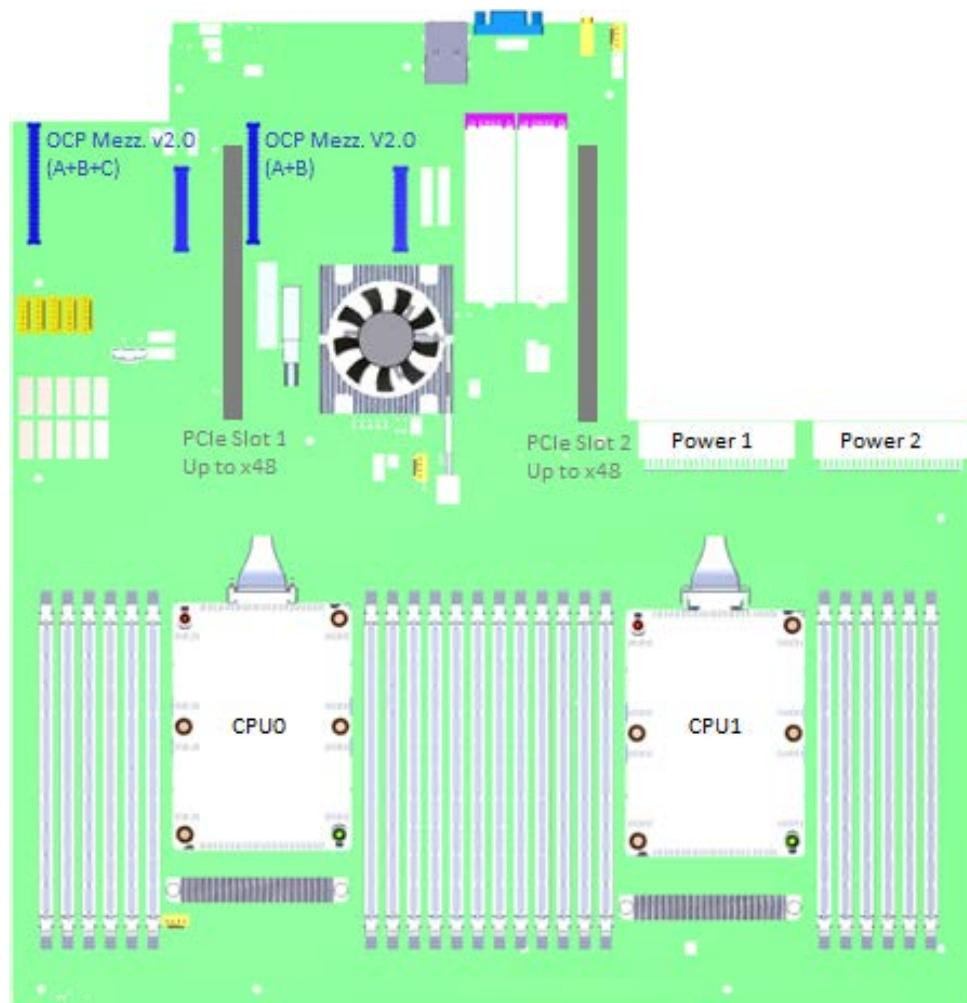
Figure 5 - Mission Peak Motherboard Function Diagram
