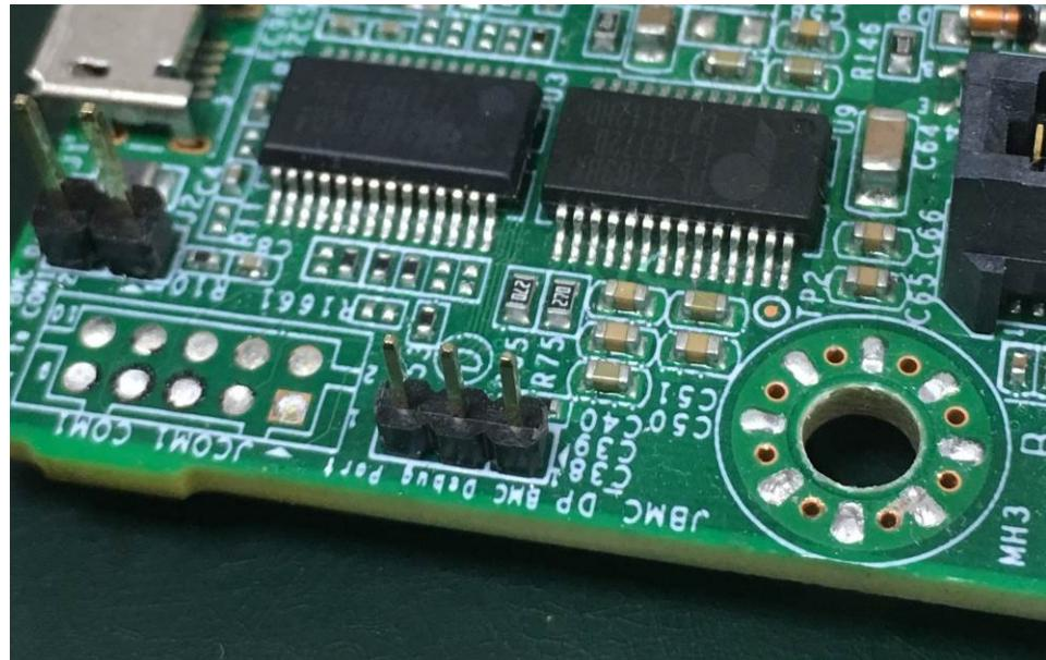
Figure 35 - JBMC Debug Header
