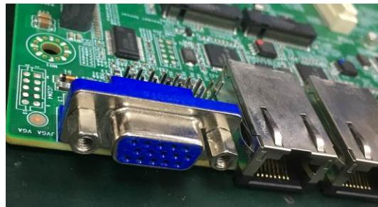
Figure 40 - VGA Header
