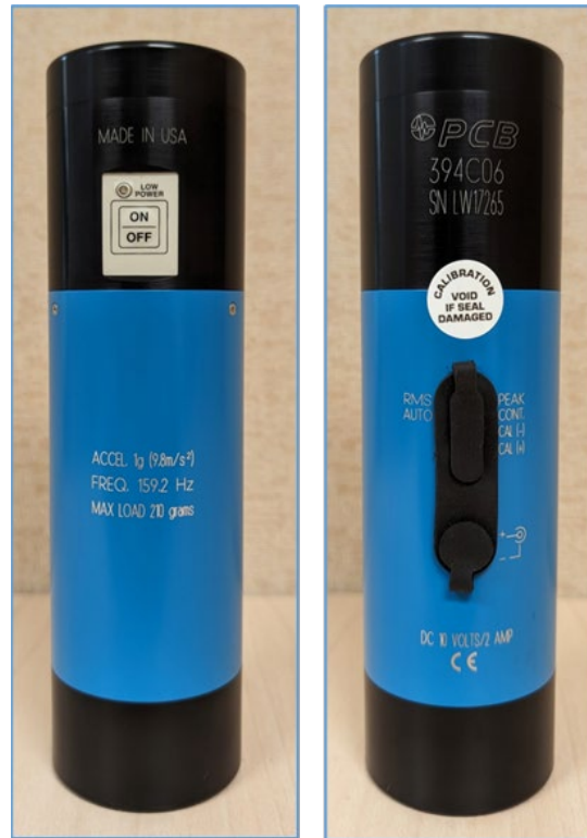
Figure 29: PCB accelerometer calibrator
