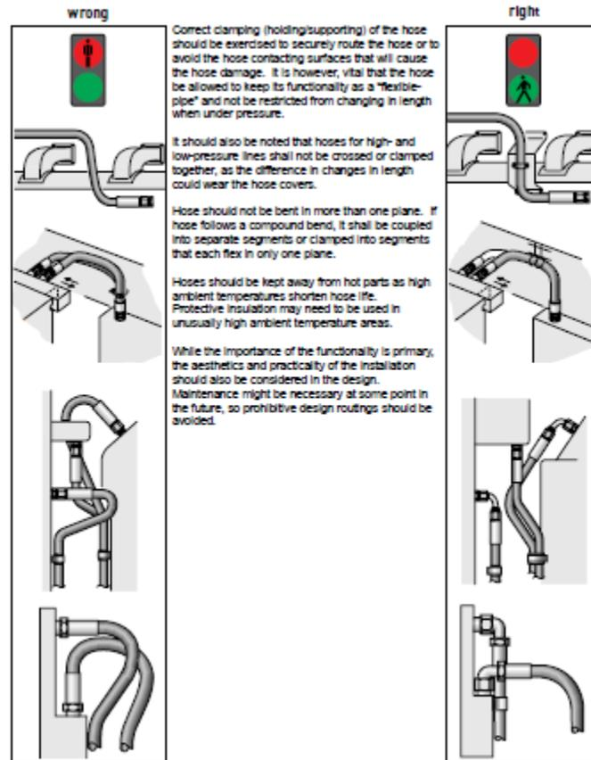
Fig. 11. Examples of proper and improper hose routing, *Hose, Fitting, and Equipment, Catalog 4400: Hose Installation Tips*, Parker Hannifin, Jun. 2017, p. E-11.
