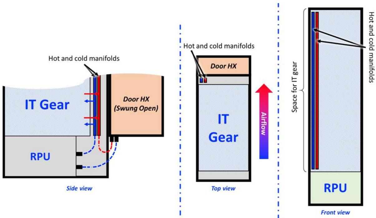
Fig. 1. Door heat exchanger mounted to a rack and coupled with RPU (or CDU) and manifolds to form a closed secondary coolant loop
