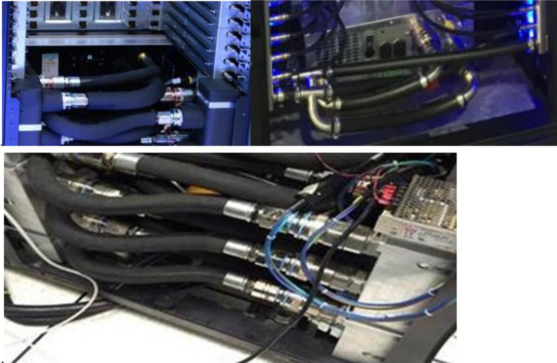
Fig. 2. Liquid Cooling Connections Using Quick Connect Couplings from Andrew Wasielewski (iPhone), *CEJN*, 3 Dec. 2015.
