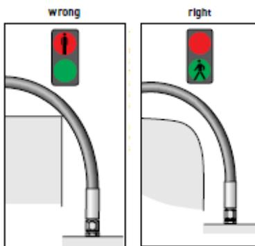
Fig. 10. Hose routing to avoid abrasion, *Hose, Fitting, and Equipment, Catalog 4400: Hose Installation Tips, Parker Hannifin*, Jun. 2017, p. E-12.
