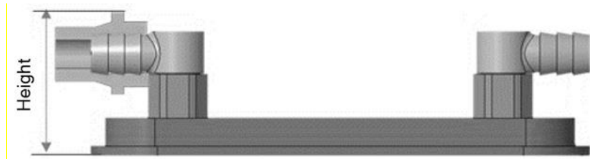
Figure 7: Diagram of the height of a cold plate
