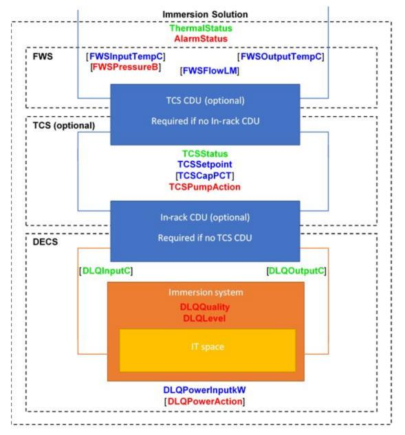
Below is an annotated example for an immersion system which is defined at CDU or integrated tank level. Shown items are the generalized items which each immersion technology should follow. Additional sensors can be added as the arrays shown below allow.
