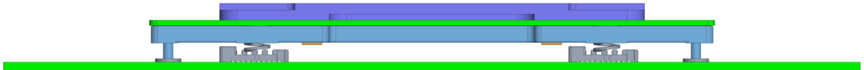
Figure 18 Side view (exploded) showing alignment pins being received by 1mm tall SMT nuts
