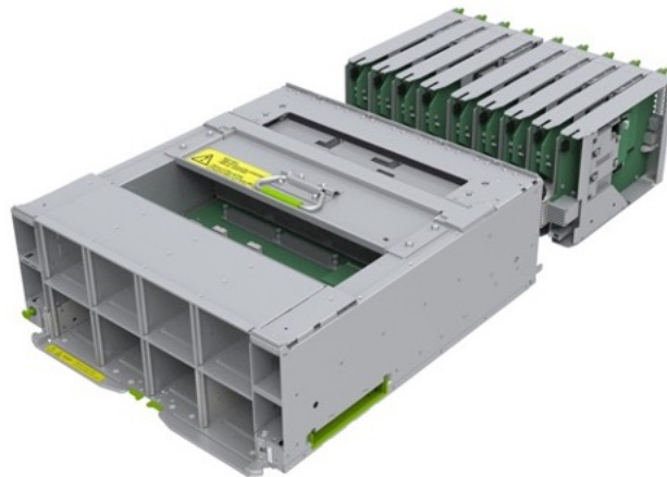
Figure 6-3: Rear ISO View of Minipack2 Orthogonal-Direct Architecture
