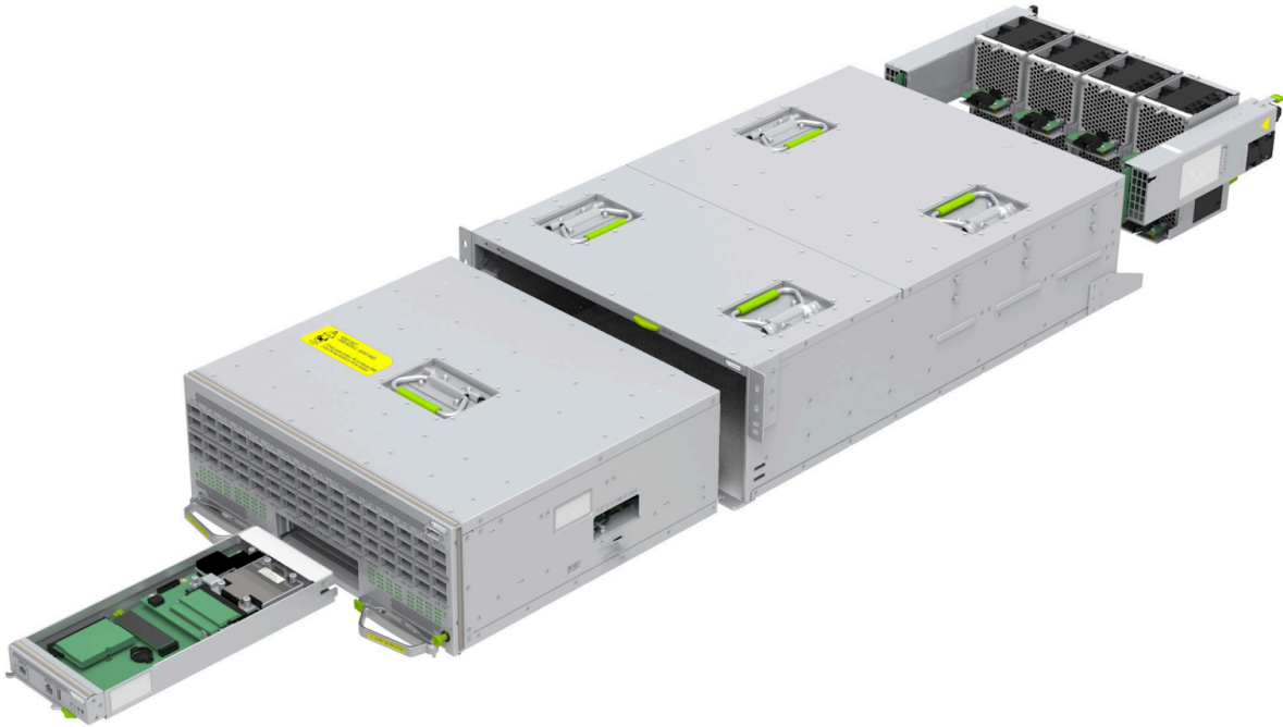
Figure 6-3: Minipack3 Chassis Exploded View
