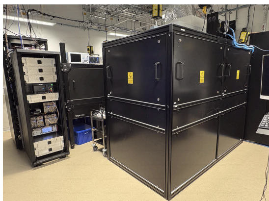
Figure 8: Neutral-atom quantum computing systems. Left: Infleqtion system deployed at a research center facility. Right: Pasqal QPU installed at Jülich Supercomputing Center in Germany
