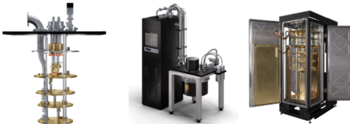
Figure 10: Examples of dilution refrigerator systems from Zero Point Cryogenics (left; Model L, and middle; Model I) and from Maybell (right; Fridge). The image on the left shows a system without user-wiring, here the upper two stages show integration of cryo-coolers. Within the middle image the cabinet shows the gas-handling system which contains electronics, pumps and storage vessels to enable the dilution fridge to operate. The right image shows a form-factor more aligned with datacenter cabinet layouts.
