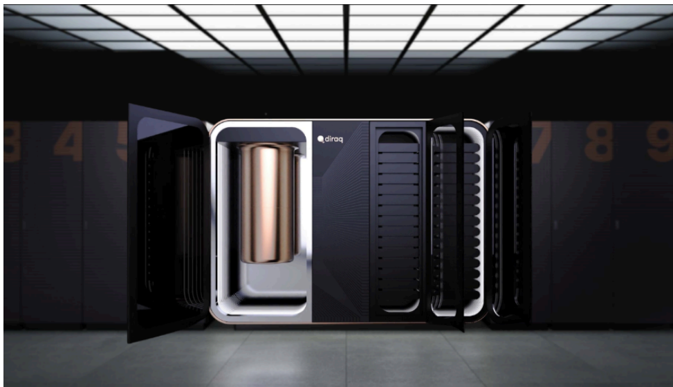
Figure 14: Artist's rendering of Diraq's spin qubit system, encompassing a cryostat, a rack of room temperature control electronics and integrated classical processing.
