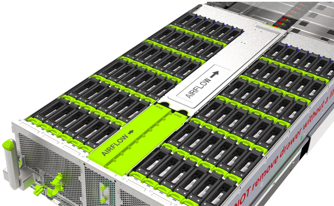
Figure 17.5: Air Baffles covering Barton Springs and SCCs
