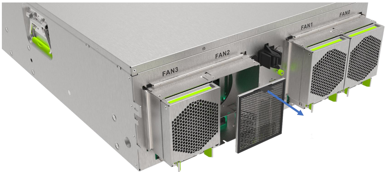
Figure 8.15: Fan Honeycomb Module Removal
