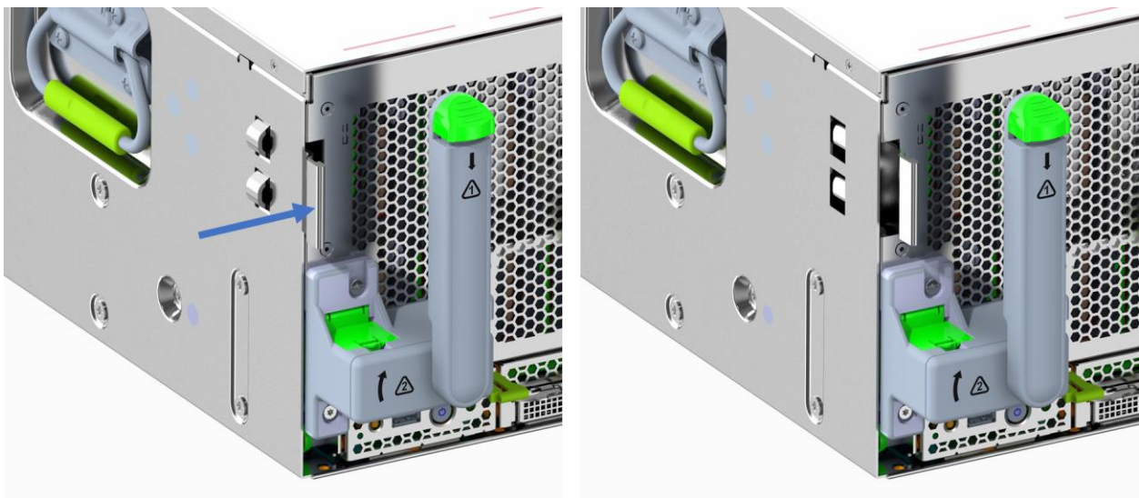
Figure 18.8: Rack Release Latch Operation
