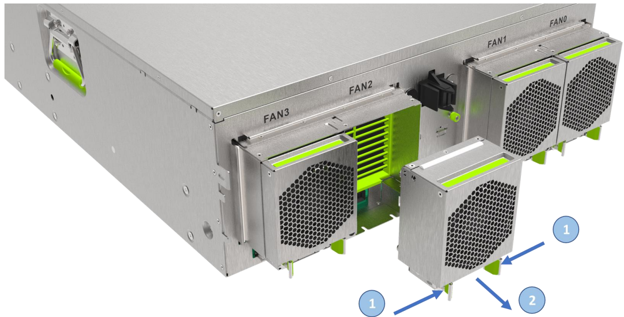
Figure 8.13: Fan Module Replacement
