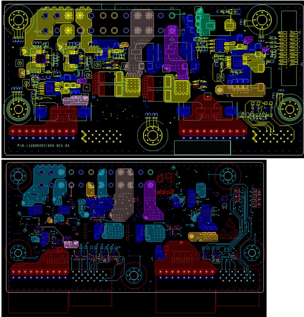
Connection board TOP/Bottom PCB Placement
