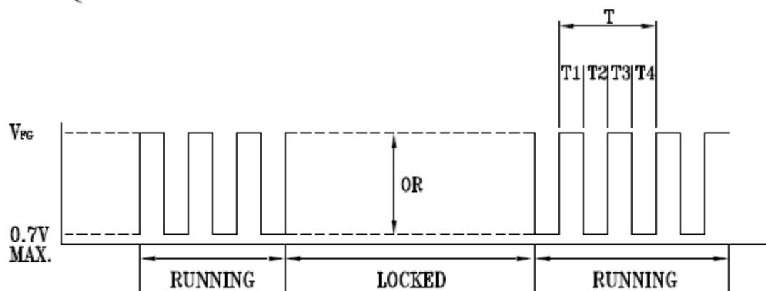
$$T = T_1 + T_2 + T_3 + T_4 = 60/N \text{ (Sec)} \quad N: \text{SPEED (RPM)}$$
