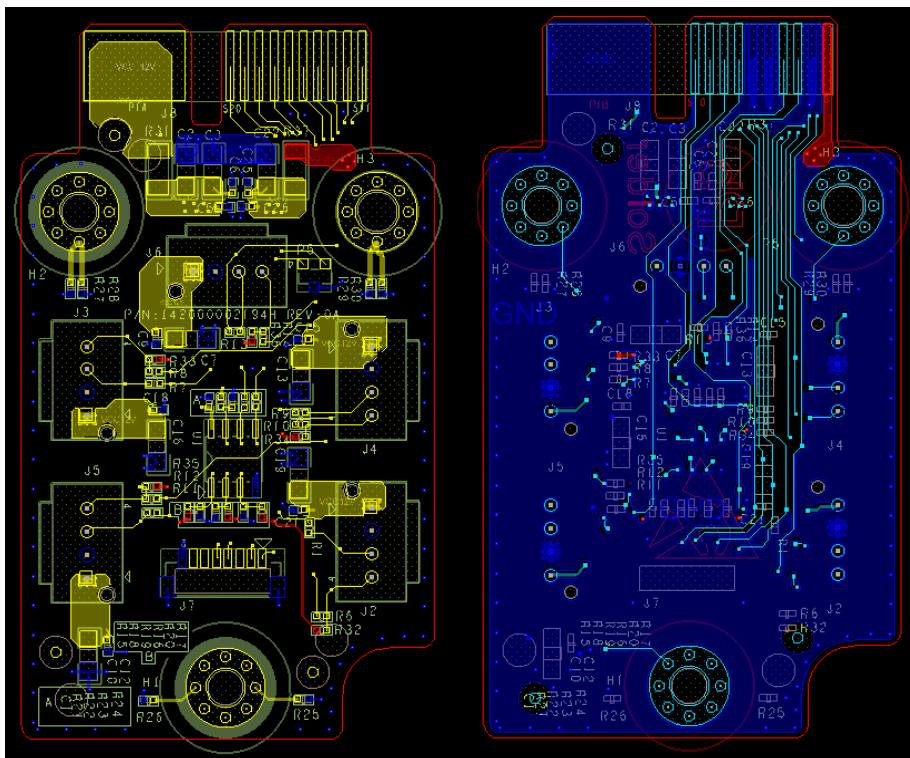
FAN board TOP/Bottom PCB Placement
