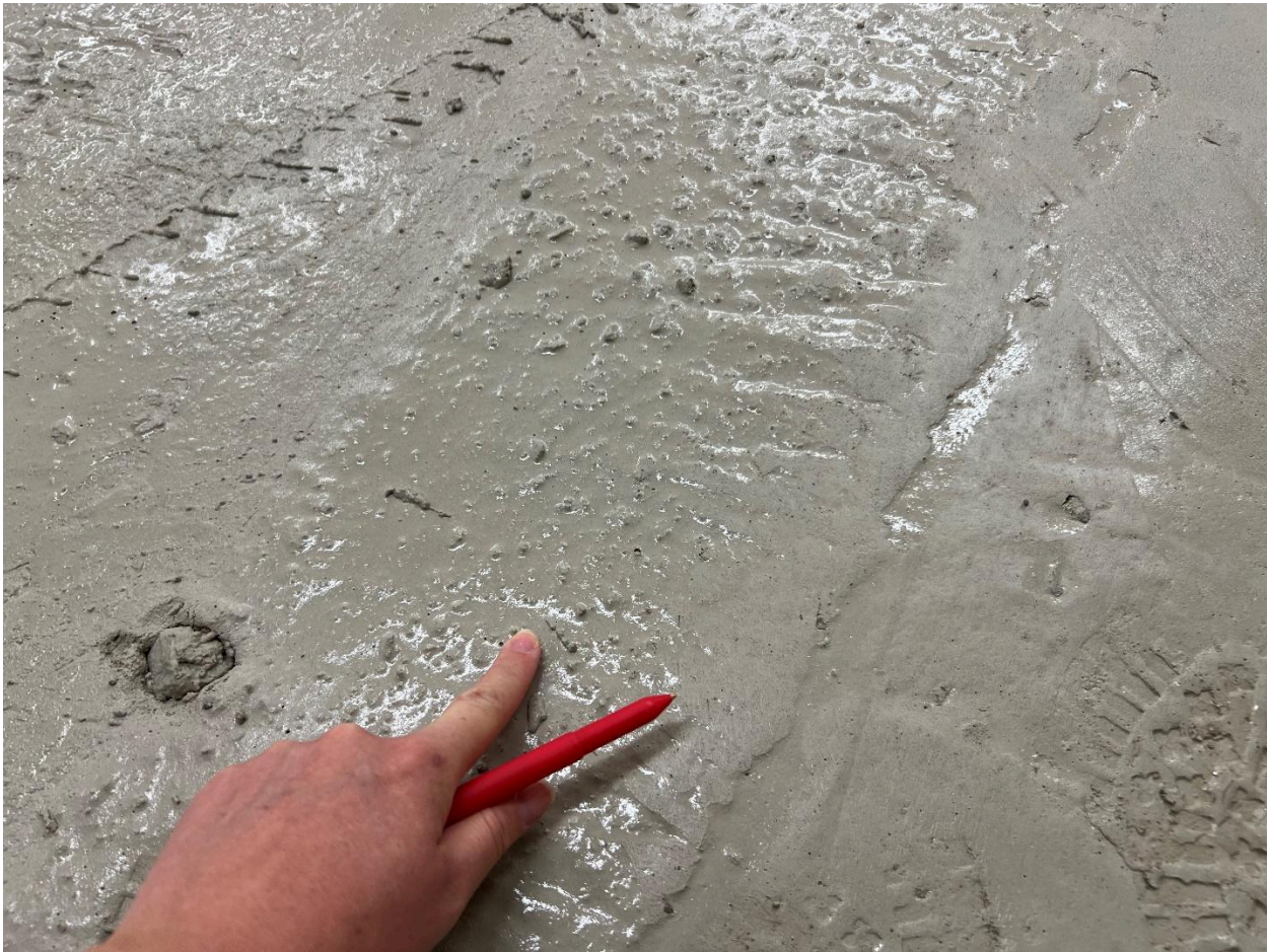
Figure 30. Slab 4, Mix 4 close-up photograph of concrete surface following placement, vibratory screeding, and bull bloating.
