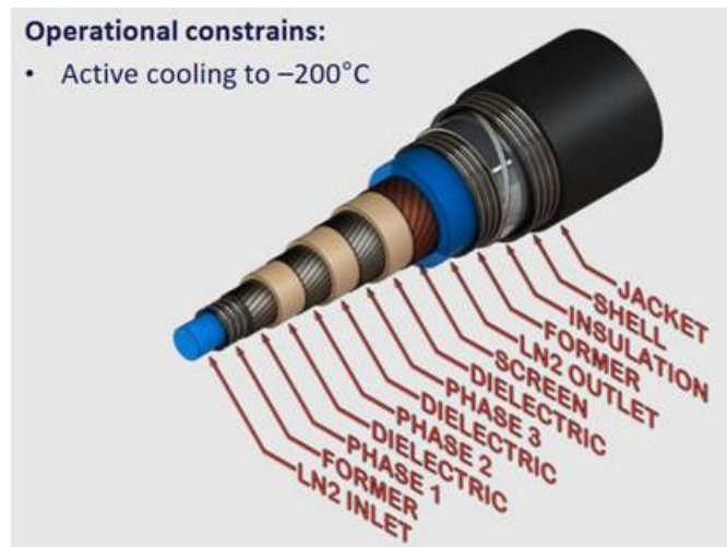
Figure 32. Superconductors Cable Cross-Section
