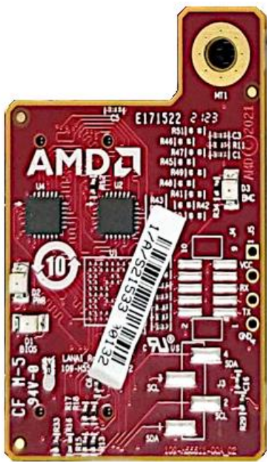
Figure 5: Lanai, Platform Root of Trust (RoT) Module
