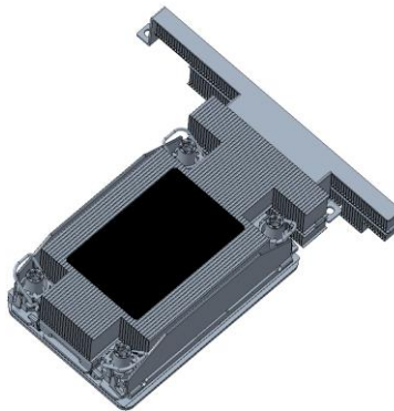
Figure 5: Open edge thermal solution for the CPU and VRMs, using an EVAC heat sink design.
