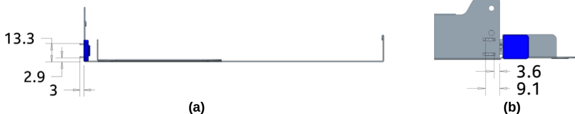
Figure 4: Basic latching dimensions for the OE sled, as viewed from the front of the sled tray (a), and in detail from the left side of the sled tray (b).
