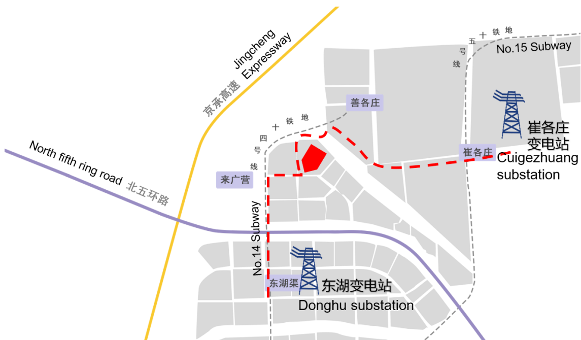
ChinData Beijing Wangjing Data Centers use two substations from different directions, which cross the Metro Line 14 and Line 15 respectively (Source: ChinData)
