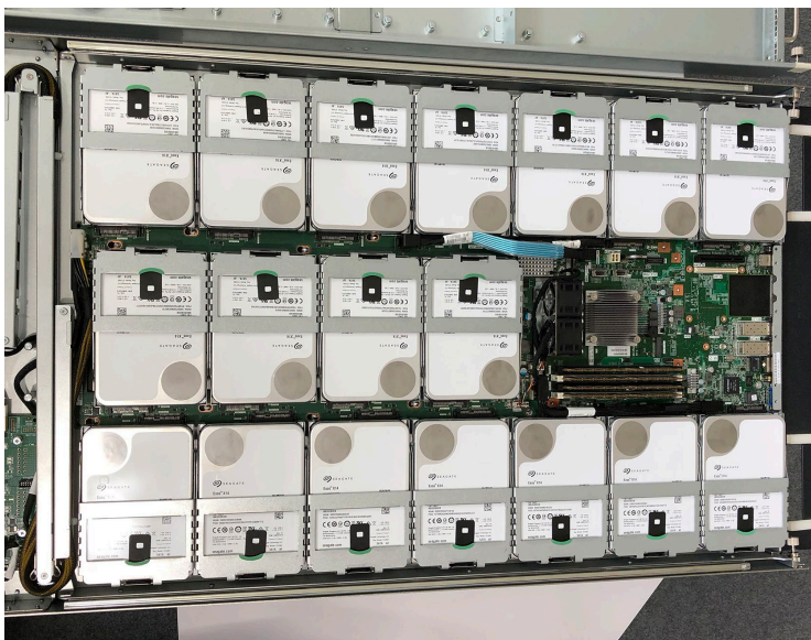
The JBOD node (only storage, used together with server head node) of Scorpio 2.5 provides 20 3.5-inch disk bays in a 1U space, and 1U can provide a bare capacity of 280TB according to its configuration with Seagate Exos X14 helium-sealed hard disk drives
