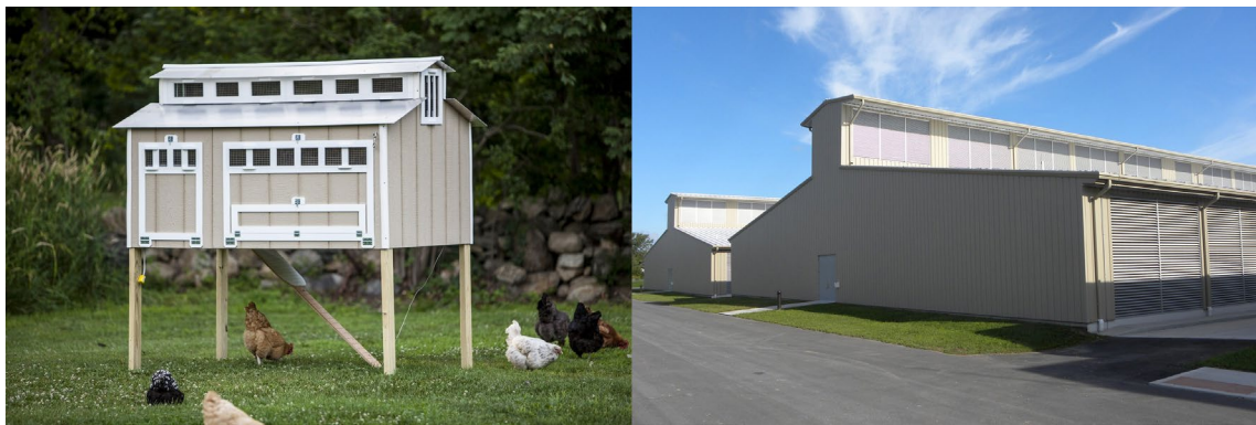
The most common grounds between the Cape Codder's chicken coop (left) and the Yahoo's “chicken coop” data center (right) are the raised attic in the middle and the louvers on both sides
